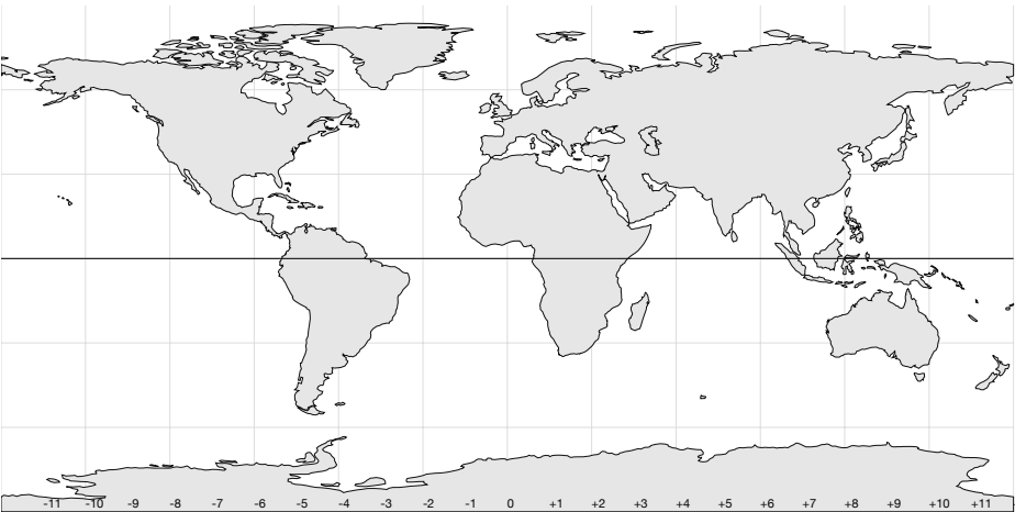
Bold line: equator. Dashed: tropics (23.44°). Figures along the foot: nominal UTC offset for that meridian. Political time zones deviate from it.
